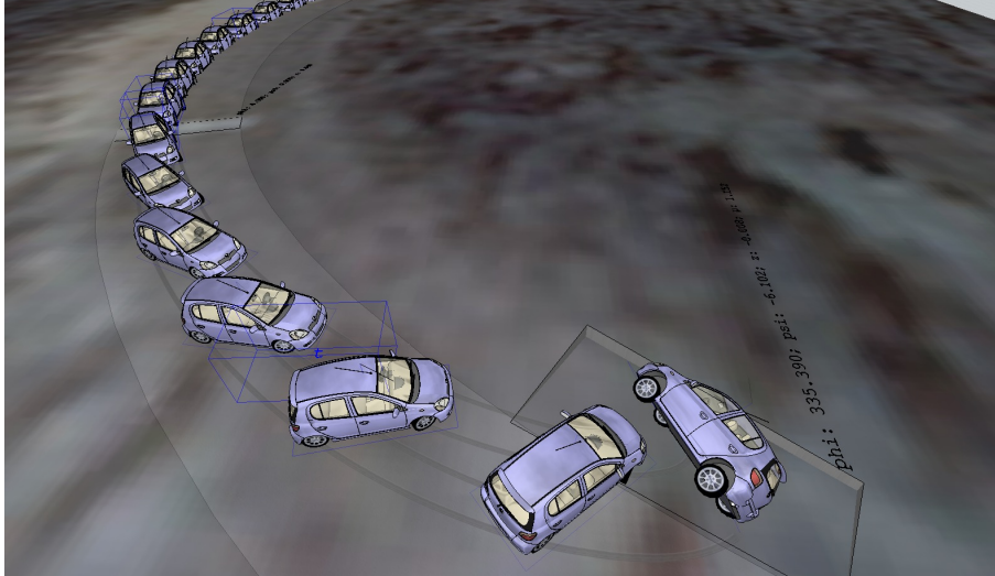
Fig. 9. The Toyota trajectory with time-separated positions (Virtual Crash 2.2)
